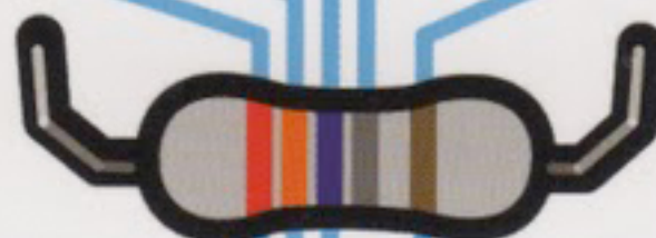
FIVE BAND (PRECISION) RESISTOR
