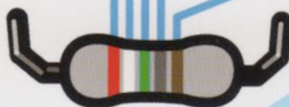
FIVE BAND (RELIABILITY) RESISTOR*
